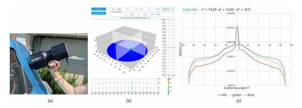
In figure (b), the 3D perspective view of the BRDF is represented. Thanks to a cross-section tool in the software, you can focus on an area of interest, such as the specular peak in this example.
