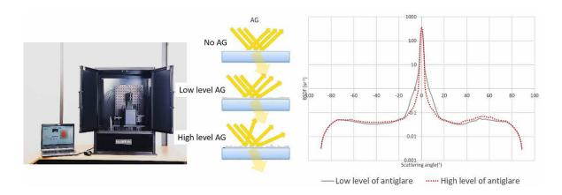
Thanks to these measurements obtained with the Synopsys Mini-Diff VPro, you can see the difference between these two levels of anti-glare. In fact, you can see that the specular peak is larger with the low level of anti-glare, which enables you to qualify the performance of this kind of screen.
