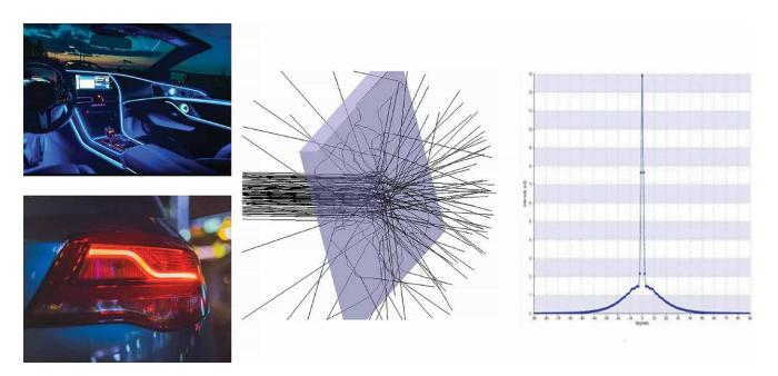
For volume scattering, we first measure the 2D BTDF of the same material in four thicknesses with the Synopsys REFLET 180S. We have developed special models in LightTools that use these four BTDF measurements to find the parameters needed to simulate the scattering of this material. You can choose either of the following volume scattering particle types:
